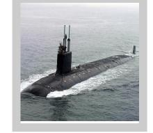
which allows the sub to glide through the water. Made of steel or titanium, sub hulls are super strong. They need to be. That's because there's a lot of pressure underwater. The deeper the sub goes, the higher the pressure becomes.
